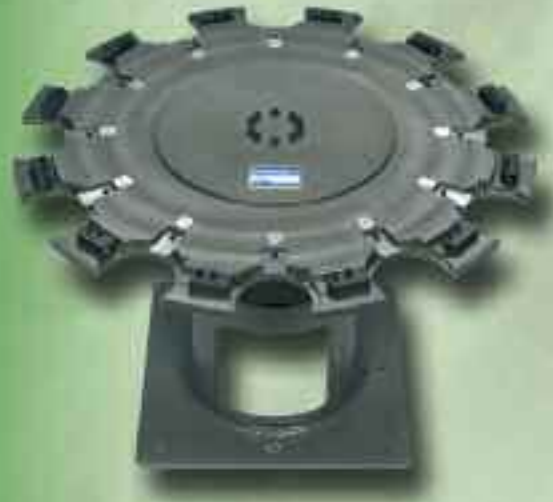
MDM050 disk magazine: equipped for SK-50 tool holder
